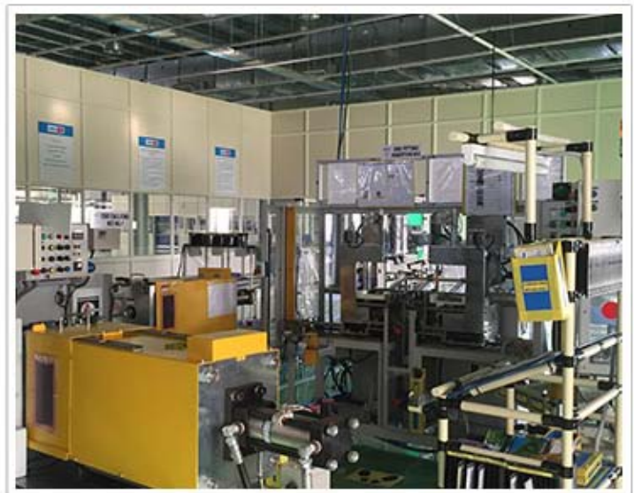
Left: Fully Automatic CHS extrusion machine for fuel hoses Right: Fully automatic Brake Hose Assembly Line
