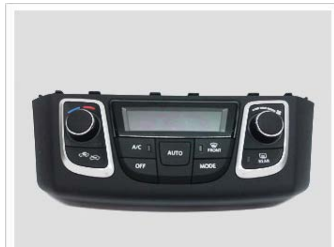
CAD View of E - HVAC Control Panel
