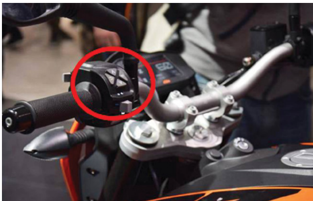
Illuminated Handle Bar Switch using Dome Switch Technology by Switch division
